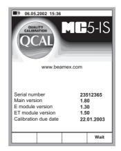
If a module's version number cannot be seen, the module is not included in the MC5-IS at hand.
