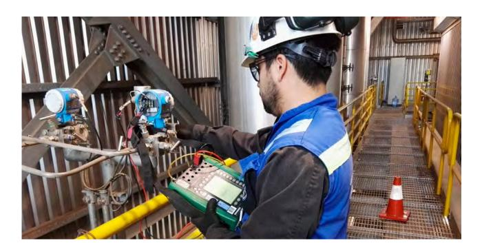
∧ MCl calibrates multi-brand transmitters for pressure, flow, level and temperature as well as switch, indicators and valves, among others.
