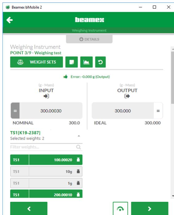
*Weighing test of a weighing instrument.*
