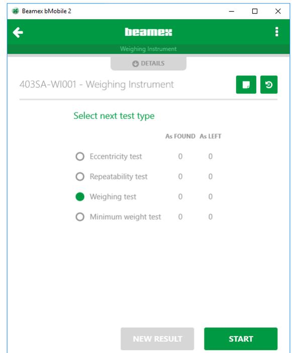
*Types of weighing tests.*
