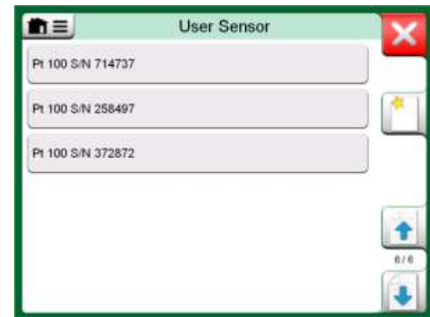
An example of a list of custom PRT sensors entered into MC6 Workstation.
