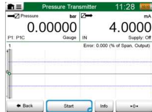
Button for zeroing a pressure module in the lower right corner.
