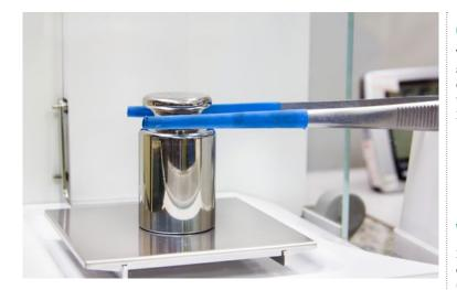
Weights should be handled so that it does not change the metrological characteristics of the weights.
