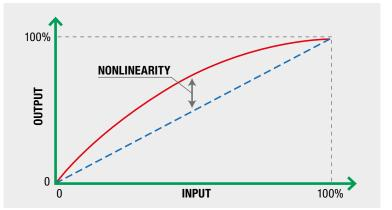
The piture above is a general illustration of unlinearity. Even instrument's zero and full range are adjusted correctly, there is error in the midrange due to unlinearity of the instrument: (SEE PIC. 2).
