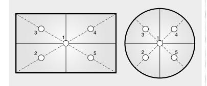
center of the load receptor (the load's center of gravity) and the result is observed. Next, the load is placed in four different sectors of the load receptor, as illustrated in the picture. (**SEE PIC. 1**)
