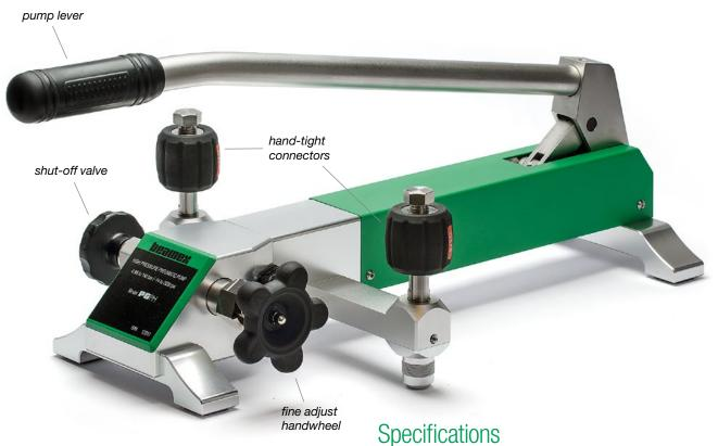
**The PGPH** is a hand-operated pneumatic (air as pressure medium) high-pressure table pressure generator. The pump is efficient in generating both vacuum and high pressure up to 140 bar (2,000 psi) quickly and effortlessly. It takes less than one minute to generate the maximum pressure. The PGPH is equipped with an adjustable volume control, providing excellent fine-tuning of generated pressure, and two hand-tight connectors allowing fast and easy connections without
