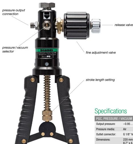
**The PGC** is a hand-operated calibration pump that can be used to generate pressure and vacuum. Using the pressure/vacuum selector you can quickly select if you want to generate pressure or vacuum. The fine adjustment provide means to accurately fine adjust the generated pressure.
