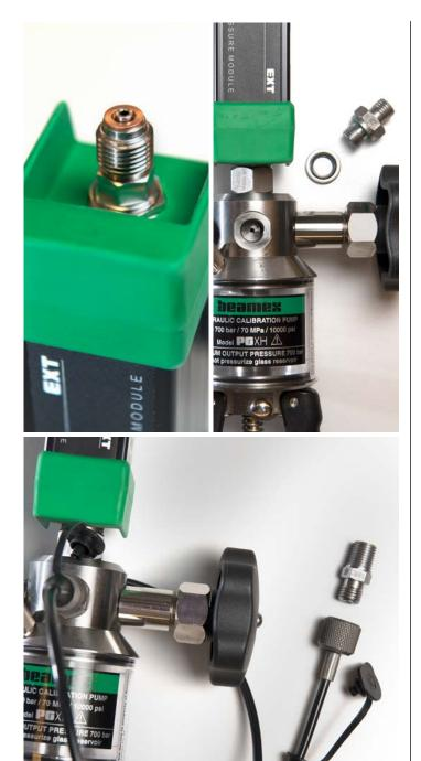
adaptor down onto the module to ensure a proper seal. If the EXT is repeatedly removed the crush washer will deform and not work properly.
