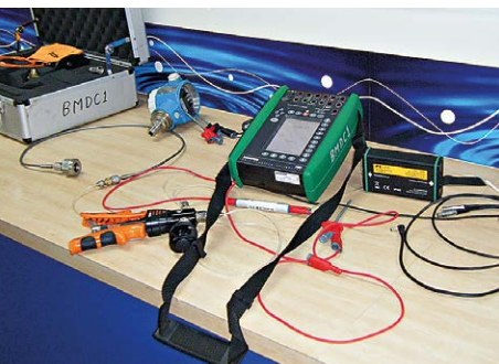
Training session on calibrating a Profibus PA E+H Cerabar S transmitter.
