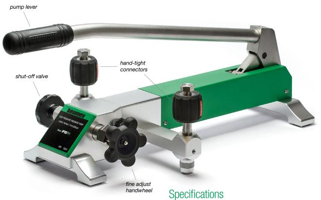
The PGPH is a hand-operated pneumatic (air as pressure medium) high-pressure table pressure generator. The pump is efficient in generating both vacuum and high pressure up to 140 bar (2,000 psi) quickly and effortlessly. It takes less than one minute to generate the maximum pressure. The PGPH is equipped with an adjustable volume control, providing excellent fine-tuning of generated pressure, and two handtight connectors allowing fast and easy connections without the need for any tools.
