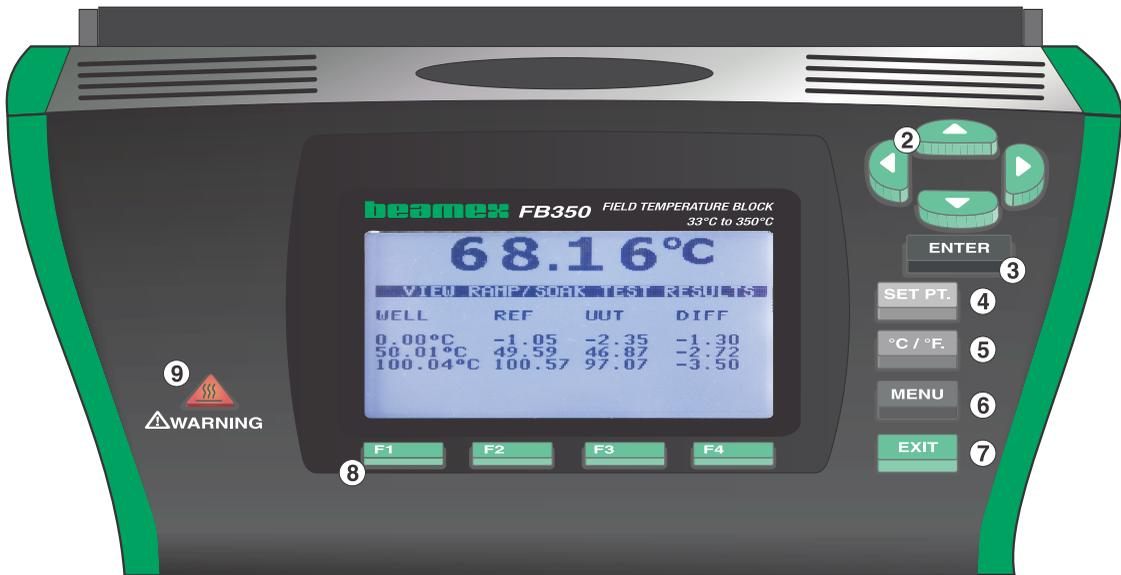
Figure 3 Display panel and keys
