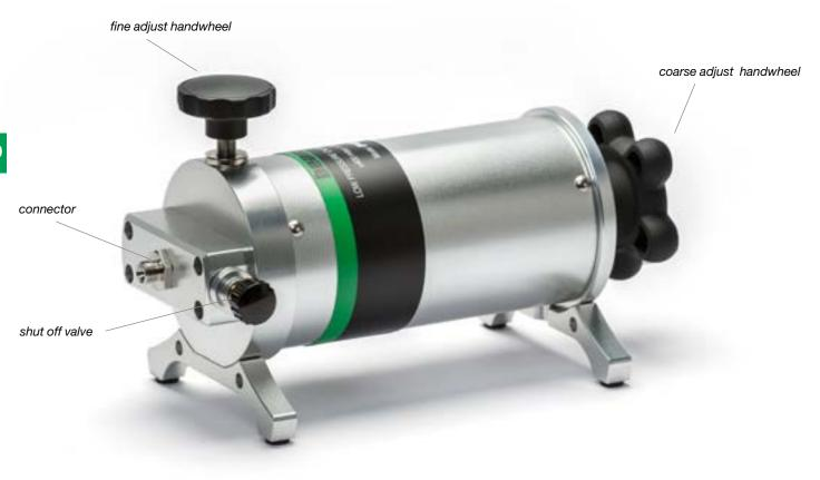
**The PGL** is a hand-operated pressure table pump for low pressure using air as its pressure medium. The pump is equipped with an isothermal bellows chamber for reducing possible environmental temperature changes during the calibration process. With the screw-operated volume control and fine adjustment, an extremely accurate and stable pressure adjustment is possible.
