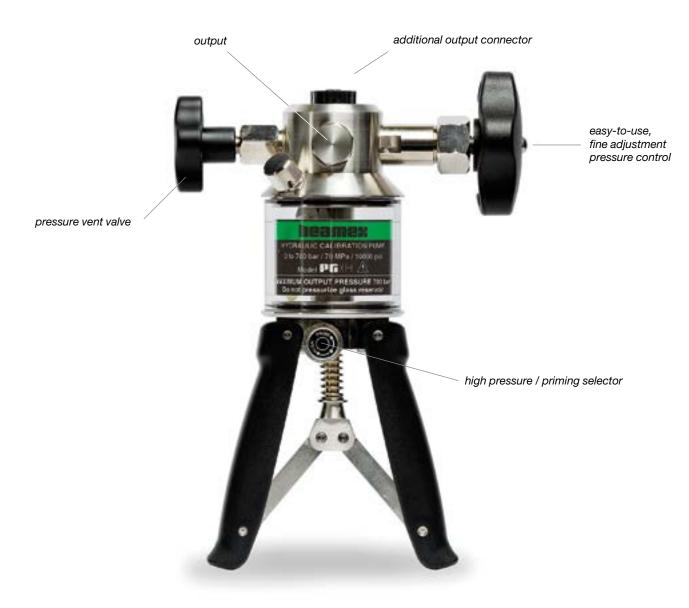
**The PGXH** is a hand-operated, hydraulic, high-pressure generator compatible with many different liquids (e.g. mineral oil, distilled water, etc.). The pump is equipped with an adjustable volume control for fine-tuning generated pressure. The PGXH can be equipped with an optional relief valve providing adjustable over pressure protection in different ranges.
