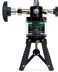
Beamex PGHH calibration pump 0 ... 700 bar / 0 ... 10 000 psi
