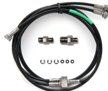
Pressure hoses 40 bar / 600 psi pressure T-hose set 1.5 m (5 ft) with NPT fittings and seals. The hoses have Bx G1/8" female threads in all ends.
