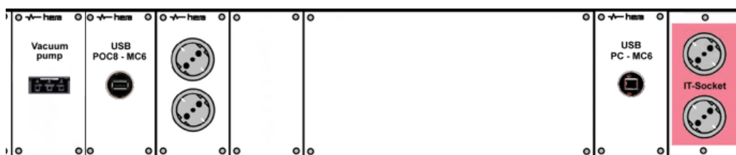
Figure 4: USB socket location – rear view of the Instrument Panel
