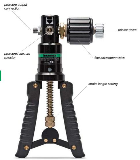
**The PGC** is a hand-operated calibration pump that can be used to generate pressure and vacuum. Using the pressure/vacuum selector you can quickly select if you want to generate pressure or vacuum. The fine adjustment provide means to accurately fine adjust the generated pressure.
