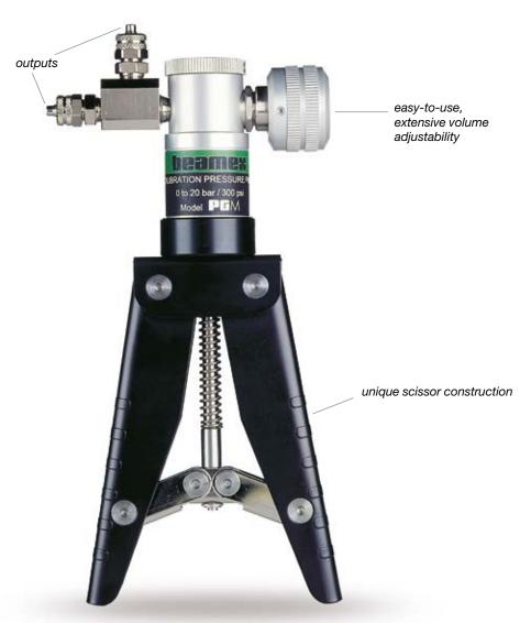
**The PGM** is a hand-operated pressure calibration pump that uses air as its pressure medium. The extremely accurate volume control provides the excellent fine adjustment of pressure. The pump's unique and sturdy construction makes the PGM the ultimate field calibration pump.
