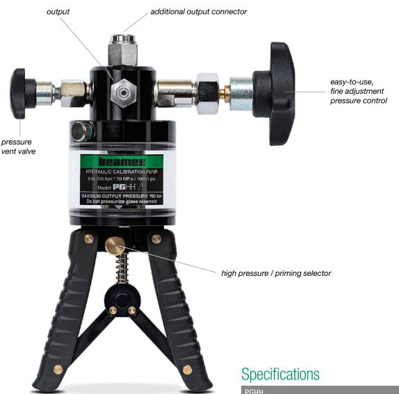
**The PGHH** is a hand-operated, hydraulic, high-pressure generator compatible with different liquids (e.g. mineral oil, distilled water, etc.). The pump is equipped with an adjustable volume control for fine-tuning generated pressure. PGHH also includes a prime/high stroke selector for easy use.
