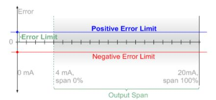
Starting from CMX V2, revision 2.7, the error can be defined as an **Error Limit Function** using two parameters:
