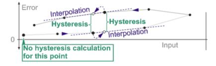
**Note:** Points where extrapolation is required to calculate the hysteresis are not taken into account.
