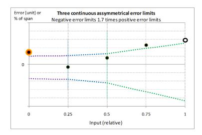
Examples of variable error limits with subranges and asymmetrical error limits:
