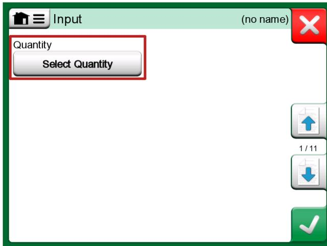
**Figure 3: Step 1: Select Quantity for the instrument Input**
