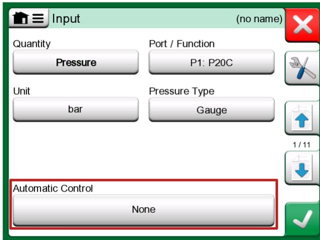
**Figure 6: Step 4: Select controller via Automatic Control**
