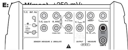
MC5-IS displays the measured low voltage in the selected window.
