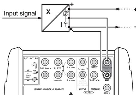
MC5-IS parallels the test diode of the transmitter and measures the externally supplied output current of the transmitter. For more information concerning test diode connections of HART instruments, see Appendix 1, chapter **Connecting MC5-IS and a HART Instrument** on page 131.
