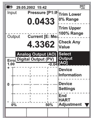
When trimming the **Digital Output** (PV), the **Input** window displays the instrument's input signal measured by MC5-IS. The **Output** window displays the digital output of the instrument.
