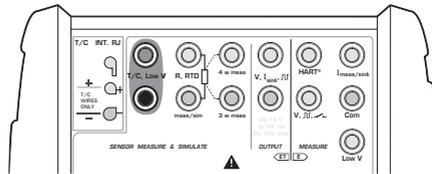
The circle indicates active terminals for each 1/**Quantity** and 2/**Function/Port** setting in the window menu.
