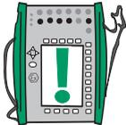
This limit switch test is a restricted version compared to the limit switch test available in Calibration Mode. This test gives you the current switch status and the approximates of the latest opening and closing points. The limit switch test in Calibration Mode offers more accurate results and additionally, statistical data of repeated switch tests. More of the Calibration Mode limit switch test in Part D of this manual.
