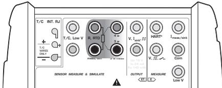
The two leftmost terminals are used in 2-wire systems. MC5-IS automatically checks the connection and displays the found wiring system (2-wire, 3-wire or 4-wire) in the measuring window. For more information concerning wiring options, see **Resistance and RTD Measurement, Connections** on page 95.
