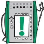
If the measured resistance value is infinite or very high (> 4000 ohm), the text “+OVER” is displayed in the measuring window. This means that the circuit is broken or the connection is wrong. Wrong connection may also cause erroneous reading, typically too low. If necessary, use the 2-wire ohm measurement to check the wiring before final connection.
