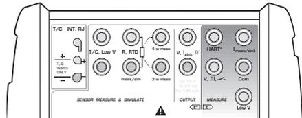
The E module also includes the optional HART modem. This allows communication with an instrument with HART capabilities. To ensure proper HART communication, make sure that the loop also includes a resistor with a resistance between 230 to 600 ohm or that the impedance of the loop itself is at least 230 ohms.
