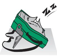
The support gives you a good viewing angle when MC5-IS is placed on a table top. Lift the support at the back of MC5-IS and place MC5-IS on the table top as shown in the picture.
