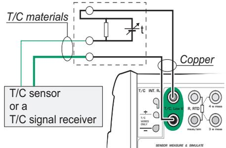
**Connection when measuring/simulating thermovoltage using a fixed temperature and Reference Junction compensation method Entered (also RJ-mode 0°C):**
