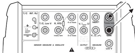
The output current of the E module is a “pure” analog signal without any embedded HART signal.
