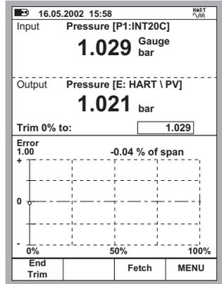
When trimming the **Analog Output** (AO), the **Input** window displays the current set point communicated by MC5-IS. The **Output** window displays the current generated by the instrument and measured by MC5-IS.
