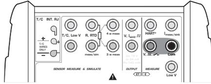
MC5-IS displays the measured voltage in the selected window.
