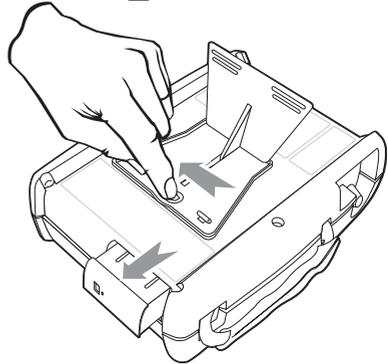
1. Turn MC5-IS upside down (the display facing the table top) and lift the support.
