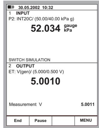
Select the Switch Type and enter the actuating point and the deactuating point of the input signal. Also enter the output signal levels for an actuated output and a deactuated output.
