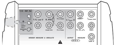
T/C measurement and simulation may also be done without the internal reference junction by using the Low Voltage terminals in the ET module. Then the reference junction arrangements have to be done outside MC5-IS and the correct reference junction settings as well as the reference junction temperature have to be informed to MC5-IS.
