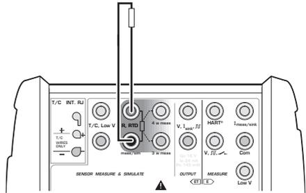
When the compensation loop wiring system is used, MC5-IS displays the text “**3-wire**”.
