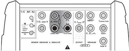
The two leftmost terminals are used in 2-wire systems. MC5-IS automatically checks the connection and displays the found wiring system (2-wire, 3-wire or 4-wire) in the measuring window. For more information concerning wiring options, see **Resistance and RTD Measurement, Connections** on page 95.
