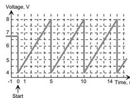
To stop ramping press the Function Key **C/Stop Ramping**. This applies for both a continuous ramping (**Repeats** field set to
