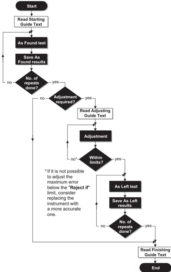
The picture gives a general view of the phases in a calibration procedure. MC5-IS supports three separate guide texts (white blocks in the picture):
