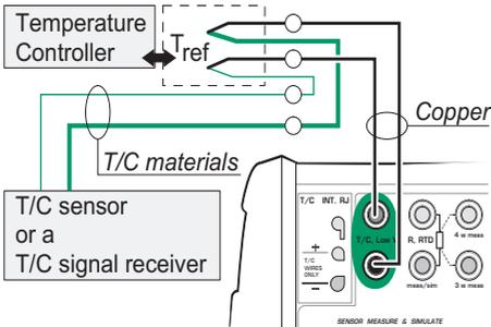
**Connection when measuring/simulating thermovoltage using a compensation box and Reference Junction compensation method Entered (also RJ-mode 0°C):**
