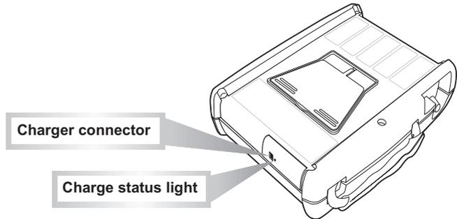
When connecting the charger, the charging electronics first checks the starting conditions. At this stage the charge status light is **green**. If the starting conditions are not met (e.g. the temperature is outside the allowed range), the status light is **blinking green**.
