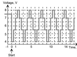
Note that because of the **Starting point** setting, the first repeat of the leftmost example is limited to a small starting step and only two full steps. Generally: if the stepping settings limit the first repeat to only a fraction of a full repeat it is still calculated as one repeat.
