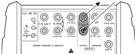
MC5-IS displays both the set value and the internally measured value for the generated voltage in the selected window. Max. output current is 1 mA.
