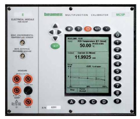
The MC5P calibration host module is, with its large graphical display and membrane keyboard, the master module for temperature, electrical and pressure calibration modules. Apart from communicating with the calibration modules, it also features communication with dry blocks and automatic pressure controllers.
