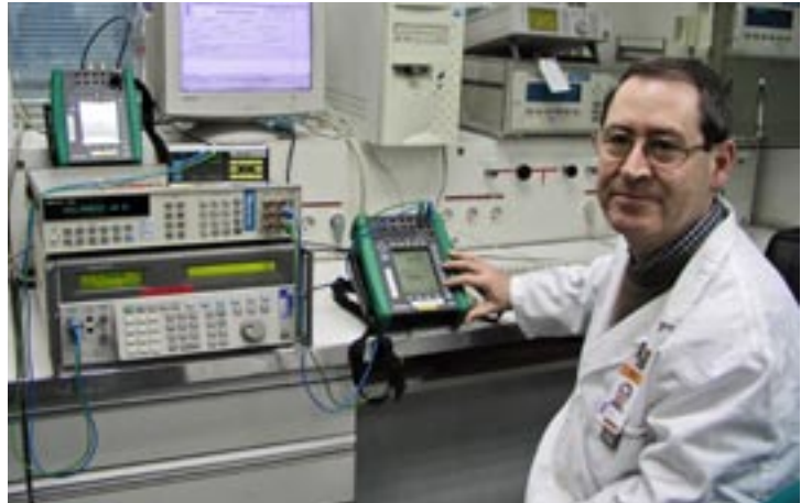
CNA has a lot of different Beamex equipment in use, such as several MC5 Multifunction Calibrators and the PG-Series of calibration hand pumps.
