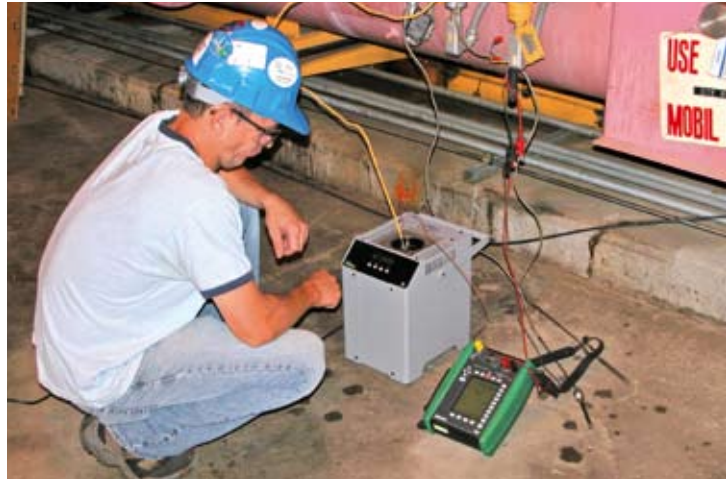
NEC’s MC5s are flexible in regards to their capabilities for calibrating pressure, temperature, and electrical and frequency calibrations.
