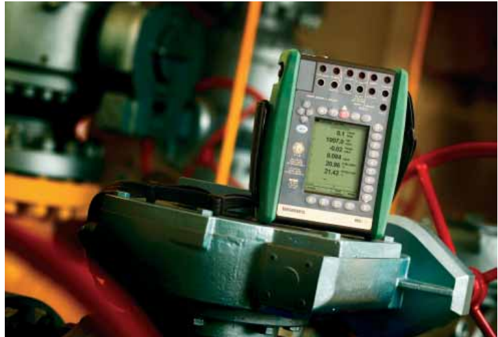
The Beamex® MC5-IS Intrinsically Safe Multifunction Calibrator was a perfect fit to the calibration needs at Łódź plant.
