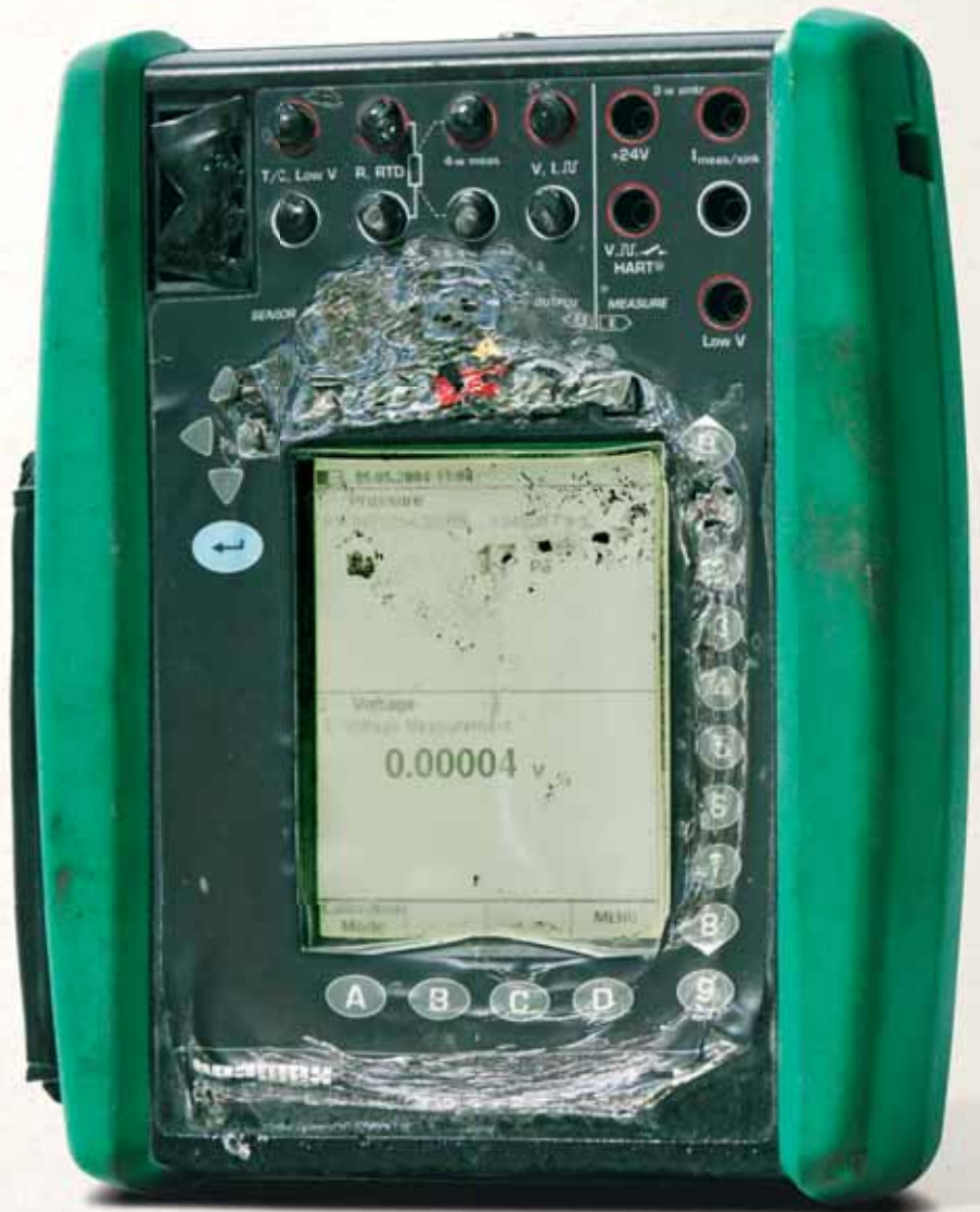
This calibrator suffered damage caused by fire, but it still works perfectly.
